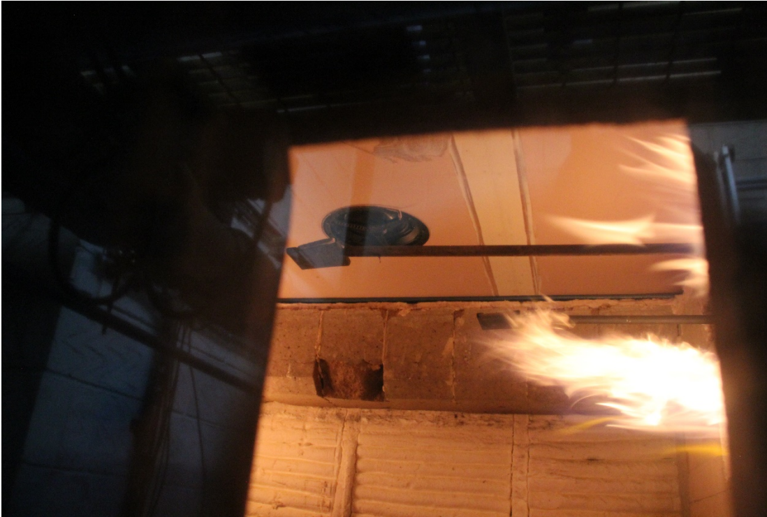
Photo 5 – 1 minute into test on exposed side where the magnetic speaker covers have fallen
